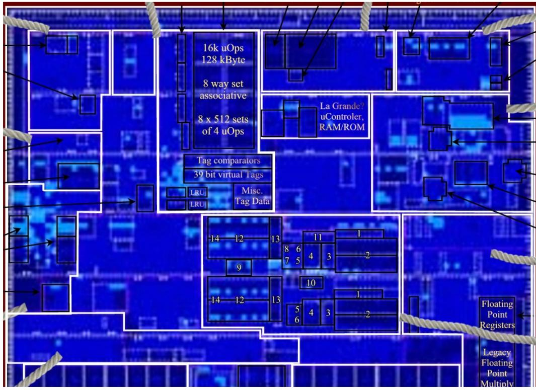
A very small fraction of the chip is used for floating-point unit.
