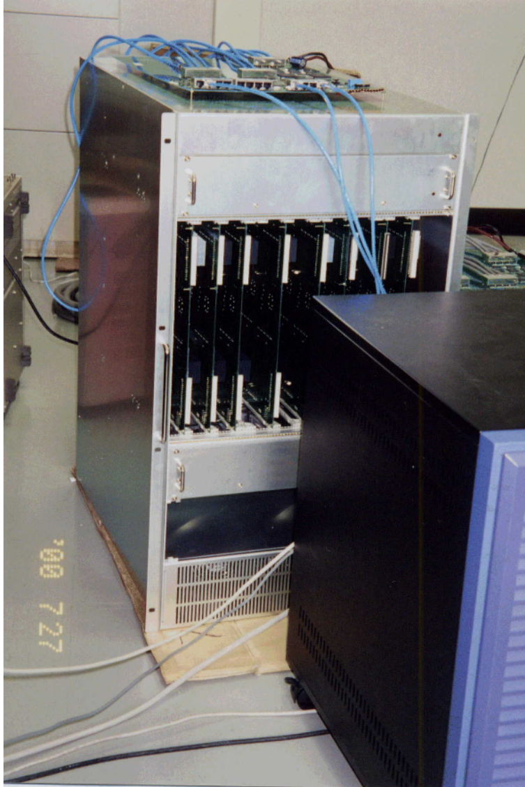
Figure 11: The six-board GRAPE-6 configuration used in this study. Eight processor boards are visible but only six were actually used in the calculation reported in this paper. The black box in front is the host computer (a two-processor Alpha box)
